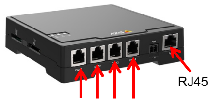
RJ12 connectors to link to 4 sensor units
