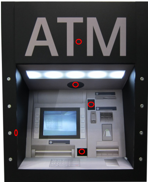
ATM (with circled areas where camera can be installed) / automated pay stations
