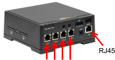
RJ12 connectors to link to 4 sensor units
